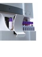
**Autoloader and STAT** 30 vacutainer tubes can be put on the autoloader for continuous loading which increases walk-away time; an independent closed tube sampler can be used for STAT test and can fit selected microtainer tubes.
